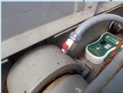
ADB Sensor Installed on Conveyor Bearing
