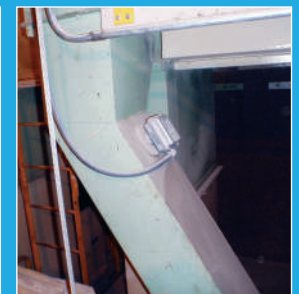
Auto-Set™ Flush Probe Installed on Belt Conveyor Discharge
